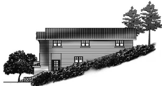
Building forms do not step down with the existing grade.
