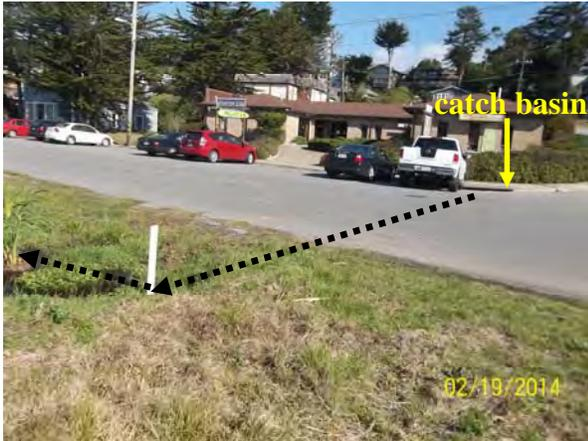
**Figure 3.** Existing catch basin at intersection of Carlos Street and California Avenue (location indicated by yellow arrow). Storm drain pipe crosses beneath Carlos Street and discharges to upstream end of Caltrans ditch that parallels Highway 1 (flow direction indicated by dotted arrow).
