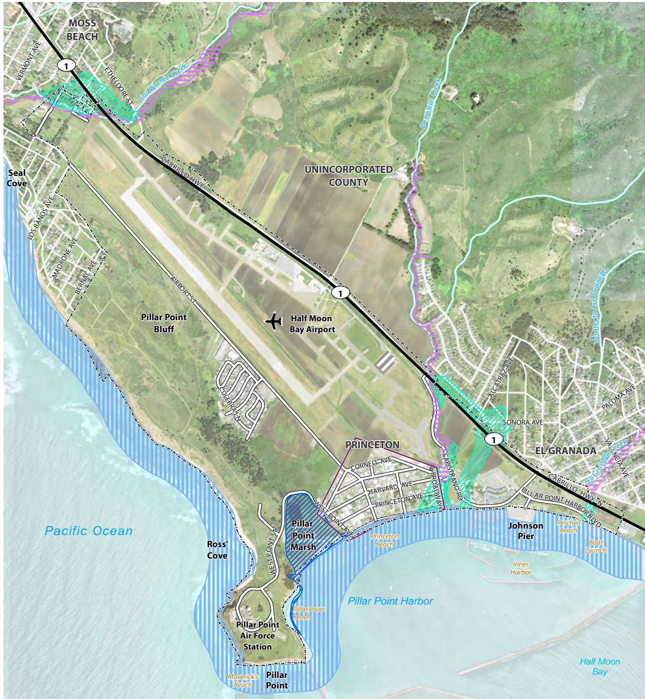
Figure 5-5: Flood Hazard Zone Map
