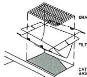
NOTE: BRING THE DISTURBED AREA TO THE GRADE OF THE DROP INLET AND SMOOTH AND COMPACT IT. APPROXIMATELY STABILIZE ALL BARE AREAS AROUND THE INLET.
