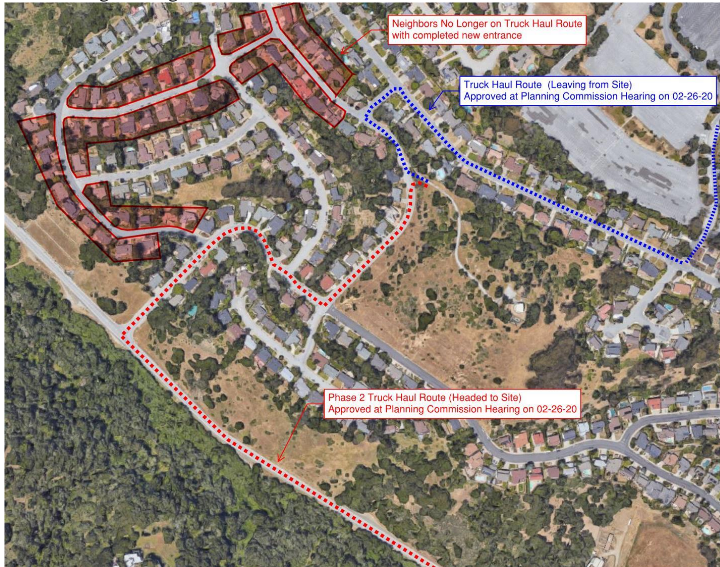
Figure 21: New entrance grading benefit to neighborhood – Trucks start using Phase 2 truck route
