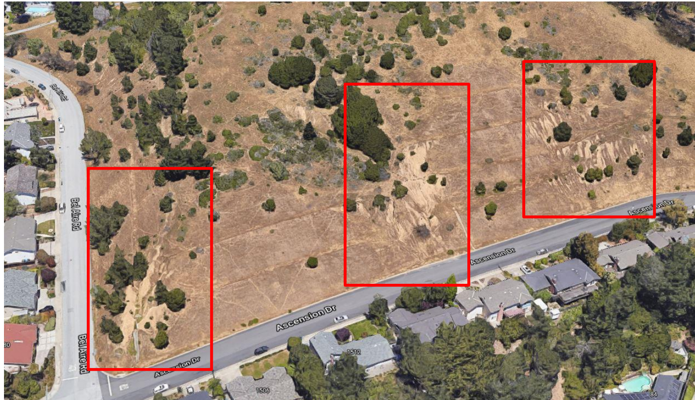
Figure 24: Ascension Drive surface erosion areas
